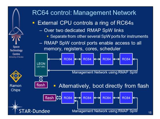
The host processor (LEON GR712RC in the slide) is in charge of boot, code distribution to the RC64 chips, monitoring their activity, collecting data on radiation events, recovery in case of faults, and security.
