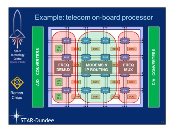
Mapping of applications to groups of RC64 ASICs is flexible, manageable by the control (host) processors, reconfigurable while in orbit
